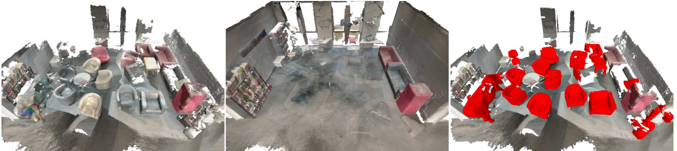
Fig. 1: Change Detection Algorithm: ( left ) One of 10 reconstructed scene observations. ( center ) Reconstruction of the static environment after 10 observations. ( right ) Discovered dynamic objects.
