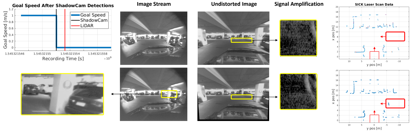
Fig. 10. Garage Experiment with DSO as the image registration method. The extended ShadowCam algorithm is able to detect the approaching car even before the front-facing LiDAR is able to detect it. This is enabled by the signal amplification relying on the registered frames within a sequence. The faint white signals on the right are visualizing how the ShadowCam can detect the approaching car based on weak illumination changes.
