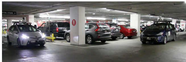
Fig. 1. Experiment with two cars. The extended ShadowCam [15] algorithm detects a moving obstacle (lights on) behind parked cars from the view point of an autonomous car (lights off) at night time driving conditions even before the LiDAR.
