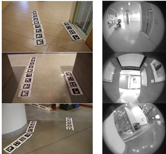
Fig. 5. Real-world corner examples. On the left side images from videos recorded with the Canon and AprilTags. On the right side images of the same corners from videos recorded with the IDS uEye and DSO. The dataset in total consists out of 7 corners.
